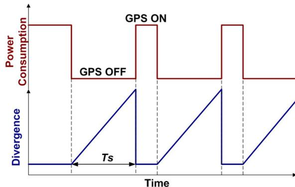
powered off the less power will be consumed by unit. Configurable parameter  $T_s$  - time the GPS module can be powered off defines trade-off between precision and power consumption.
