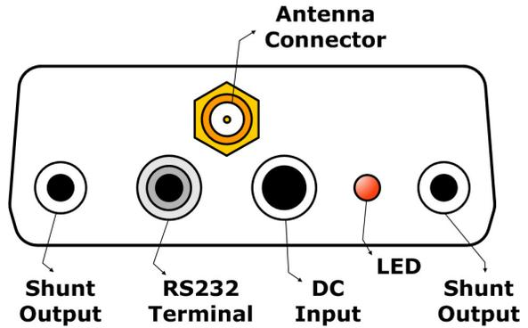
**RS232 Terminal** output is used to connect interX to PC RS232 port. Additional information about interX RS232 terminal can be found in Section RS232 Terminal .
