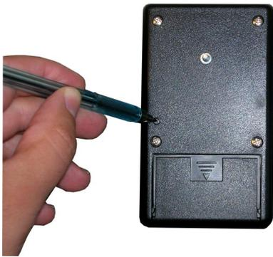
To turn interX on press button for at least 4 seconds
