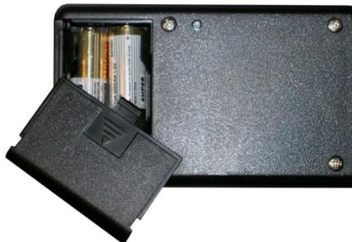
On bottom side of interX there are battery holder compartment and on-off push button.
